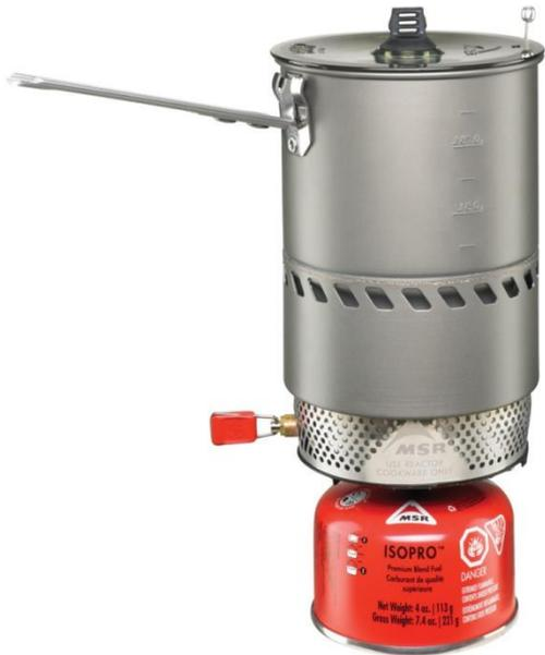
The gas contained in the canister is a blend of propane and either butane or iso-butane. There are two major reasons for using a blended gas. Butane is more stable than propane at ambient temperatures, which allows the gas to be safely stored in a lightweight canister, as opposed to the heavy-duty steel tanks required to safely store pure propane.
